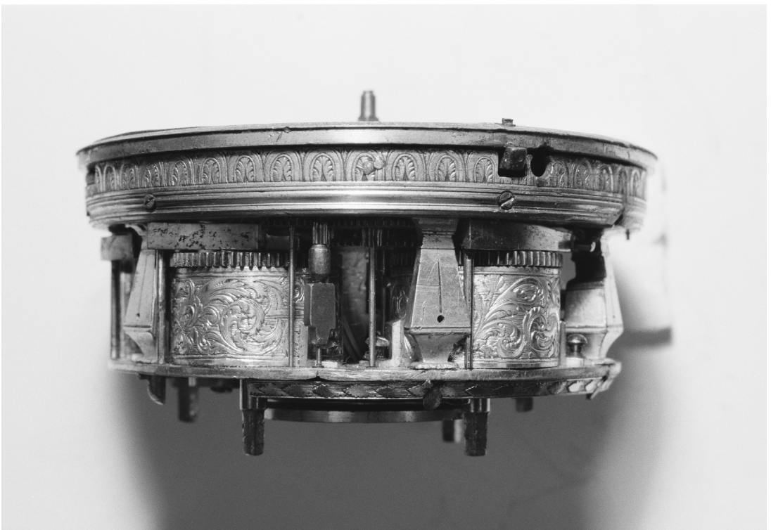
Above: view of the Zeidlmaier watch movement. Below: the decorated rim, the pillars and the engraved barrels are visible in this side view. (Both photos Deutsches Museum, photographer unknown.)
